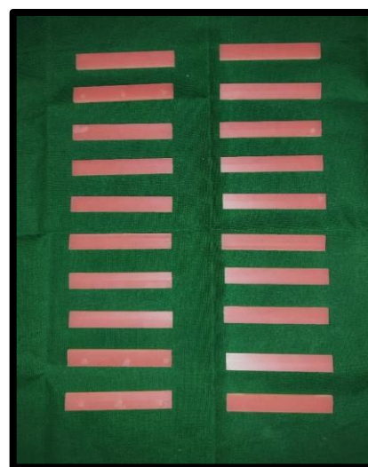
FIG 5: Group 2- 20 pre-polymerized pink PMMA Ivotion base CAD-CAM Milled specimens
